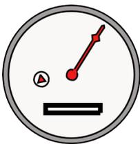
Newer meters have a red or black triangle and a needle that moves when water is flowing through the meter. Watch this to detect a leak.
